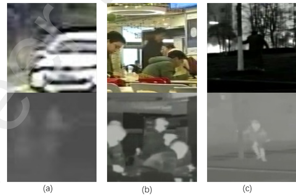
Figure 1: Complementary image between two modes. (a) shows that visible information is dominant. (b) shows that both modes are important. (c) shows that infrared information is dominant.
